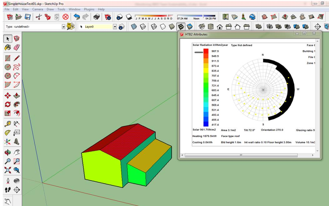
To import an EnergyPlus weather file in to the VirVil Sketchup Extension, go to > Extensions > VirVil > Tools > Add HTB2 files Attributes, a new small window will appear, click on the “EPW” file you require and press Open. VirVil will convert the file into a HTB2 Weather file ready for use in your modelling.
