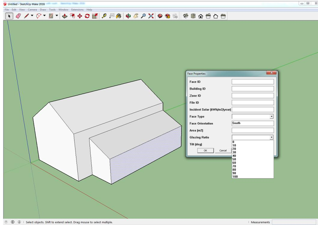
Select faces to set the glazing ratio or correct the face type. Just right click the face and open the window of face properties, then input the glazing ratio for that façade or roof. The default glazing ratio is 50%.
