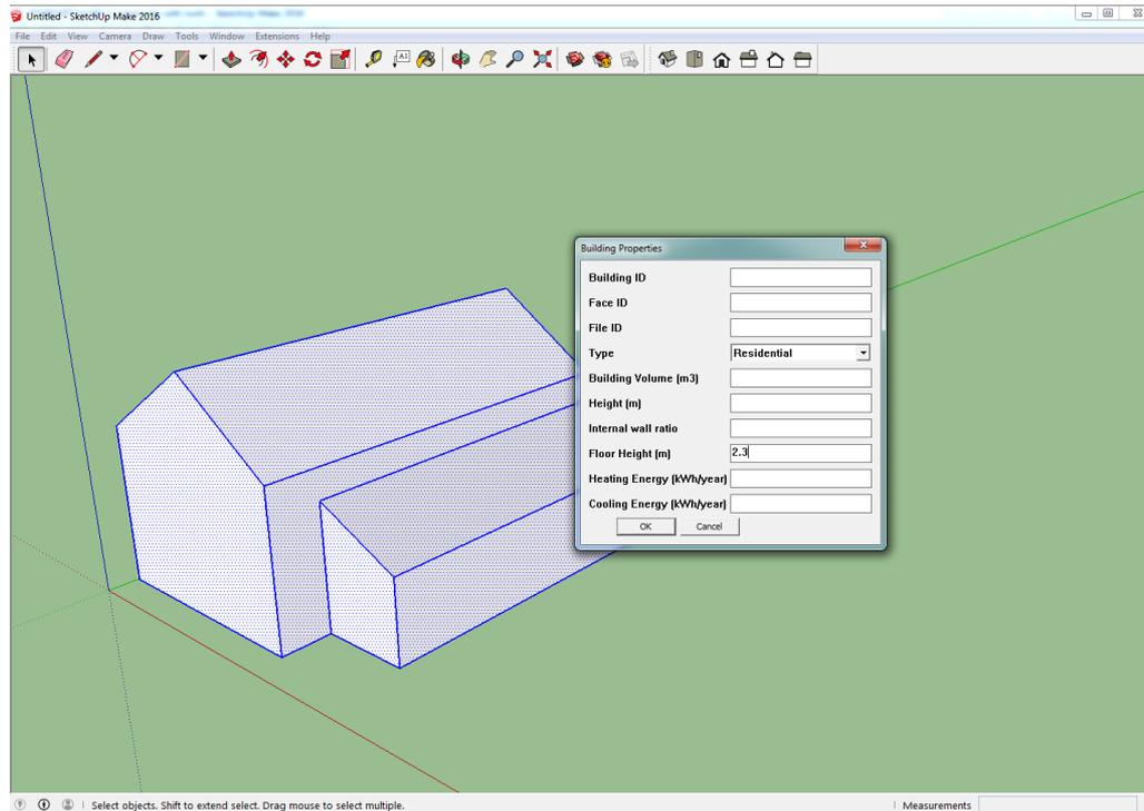
Triple click to select the whole building, then right click and open the window of Building properties, select the building type, and input the floor height. The default building type is residential, and default floor height is 3m.
